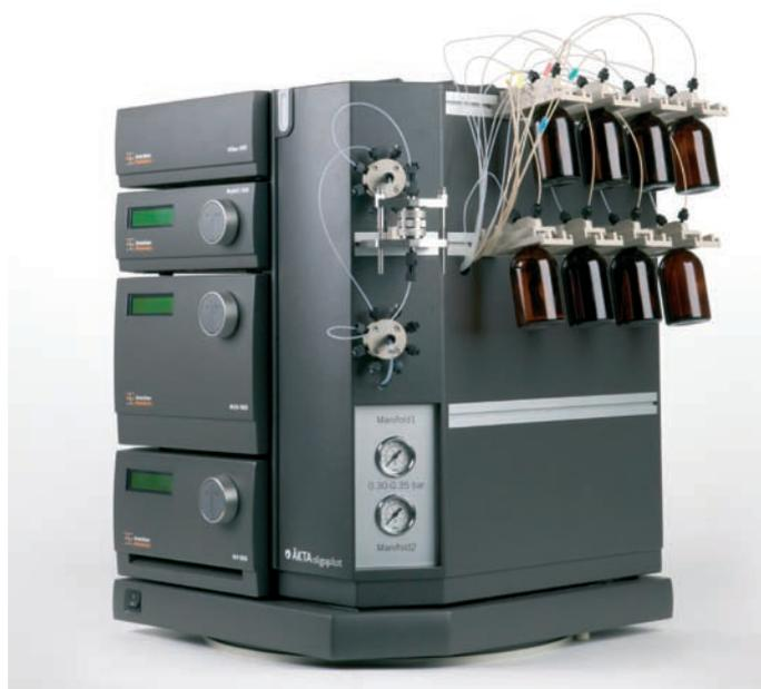
**Fig 1.** ÄKTA oligopilot 100 was used for the initial optimization and initial scale-up to 380  $\mu\text{mol}$ .
