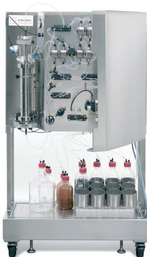
Fig 2. OligoPilot 400 was used for the final scale-up to 1.52 mmol.
