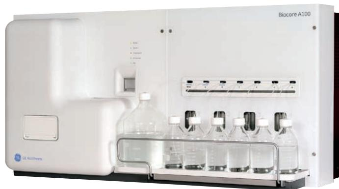
**Figure 1.** Biacore A100 provides label-free analysis of interactions for selectivity-based compound screening.
