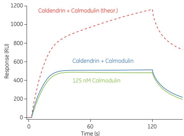
**Fig 8.** Competition analysis between calmodulin and caldendrin binding to AKAP79. Calmodulin was injected in the presence (red) and absence of caldendrin (blue). The red dashed curve is a simulation of the theoretical signal under non-competitive conditions. Experimental analysis was performed using a Biacore S51 system.
