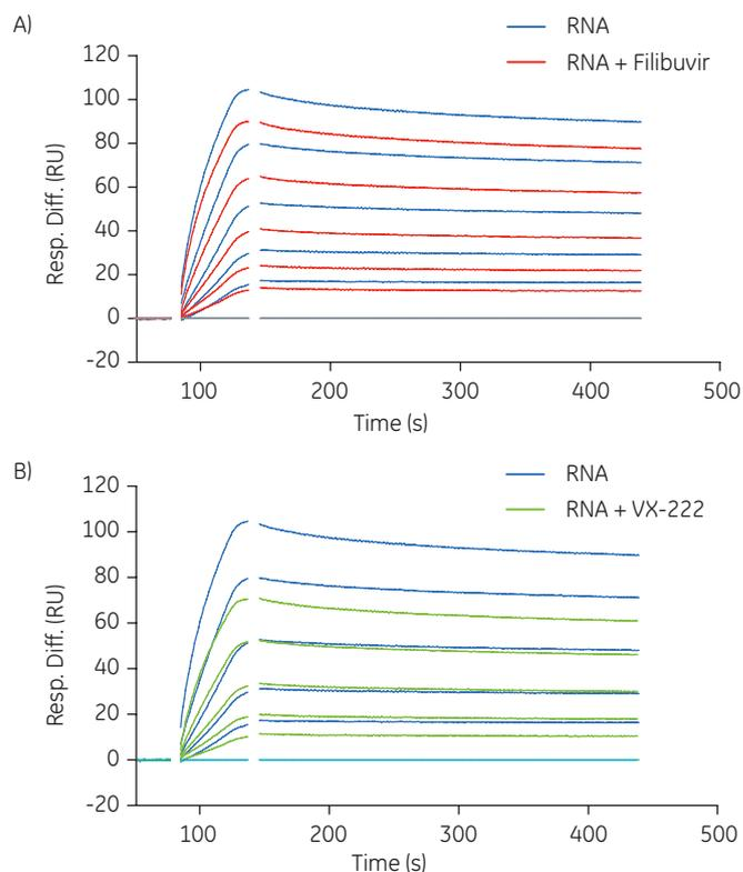
**Fig 4.** Sensorgrams representing the interaction between immobilized HCV polymerase and RNA in the absence and presence of inhibitor. (A) RNA in the absence and presence of 300 nM filibuvir. (B) RNA in the absence and presence of 300 nM VX-222. RNA concentrations were 8, 4, 2, 1, and 0.5  $\mu\text{g/ml}$ . Sensorgrams are blank and reference subtracted.
