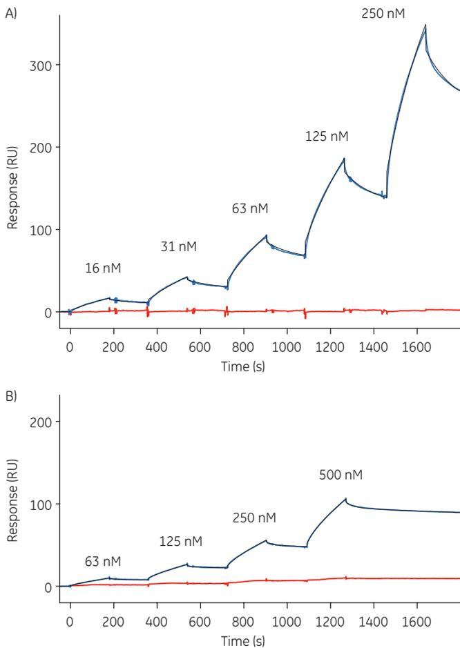
**Fig 7.** Sensorgrams showing single cycle kinetic analysis of AKAP79 interactions with A) caldendrin with calcium B) caldendrin without calcium. Red curves show a negative control analyzed under the same conditions. Overlaid black lines represent theoretical best fit sensorgrams using a 2-state interaction model.
