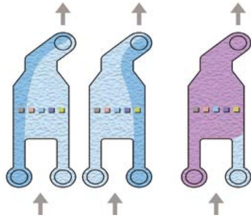
**Figure 7b.** i) Immobilization of interactant to spot 1 ii) Immobilization of a different interactant to spot 5 iii) Sample flows over all spots simultaneously.
