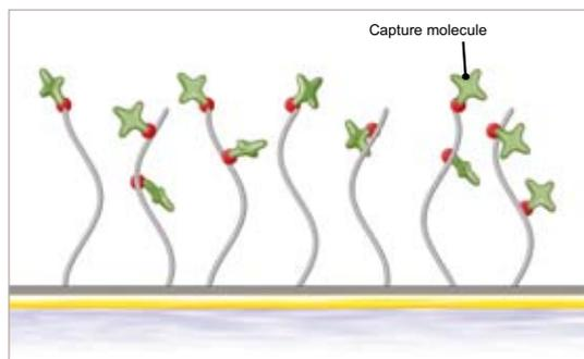
**Figure 10B.** An example of a sensor surface designed for immobilization of interacting partners via a capture molecule.
