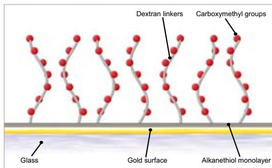
**Figure 10A.** An example of a sensor surface designed for direct, covalent immobilization of interacting partners.
