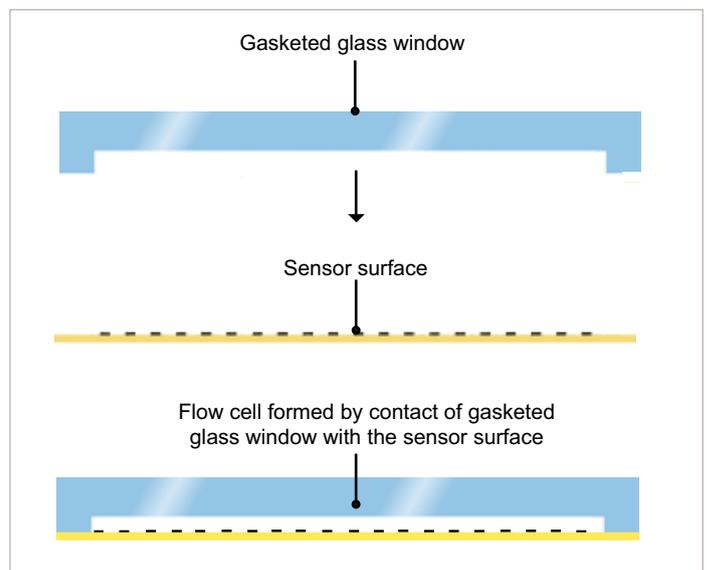
**Figure 4B.** Flow cells are formed in GC-SPR by hermetically sealing a gasketed window with an inlet and an outlet valve over the sensor surface.
