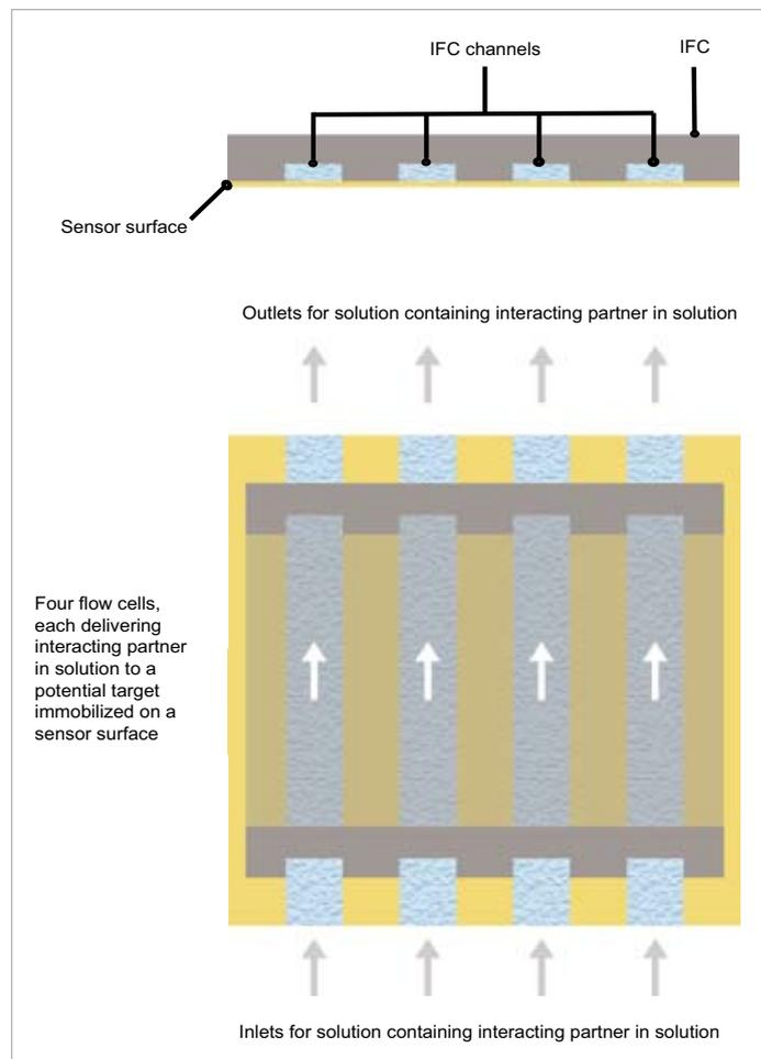
**Figure 6.** Independent flow cells for concentration analyses.
