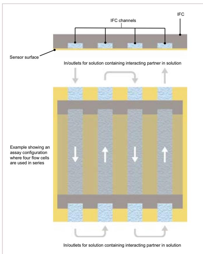
**Figure 5.** Flow cells in series in which selected cells may be used for on-line referencing, allowing direct background subtraction for accurate kinetic analyses
