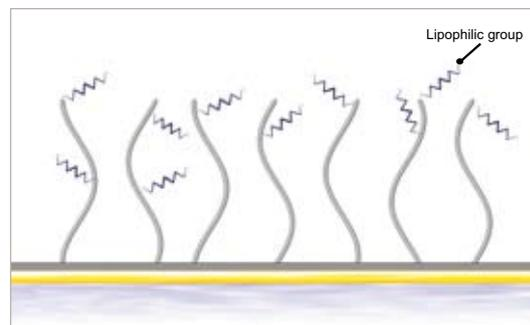
**Figure 10C.** An example of a sensor surface designed for immobilization of hydrophobic interacting partners such as liposomes or membranes.
