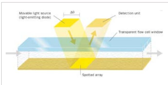
**Figure 3.** GC-SPR. Sample is injected through a single broad channel and interacts simultaneously with all spots on the array.
