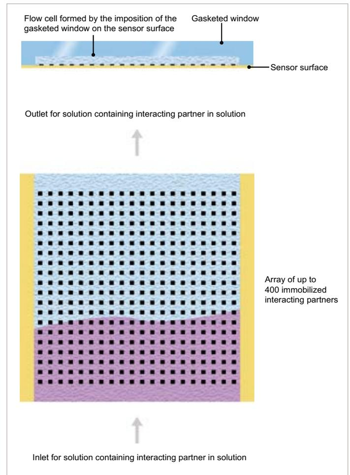
**Figure 8.** Single pass, multi-spot flow cells for simultaneous profiling of up to 400 interactions.
