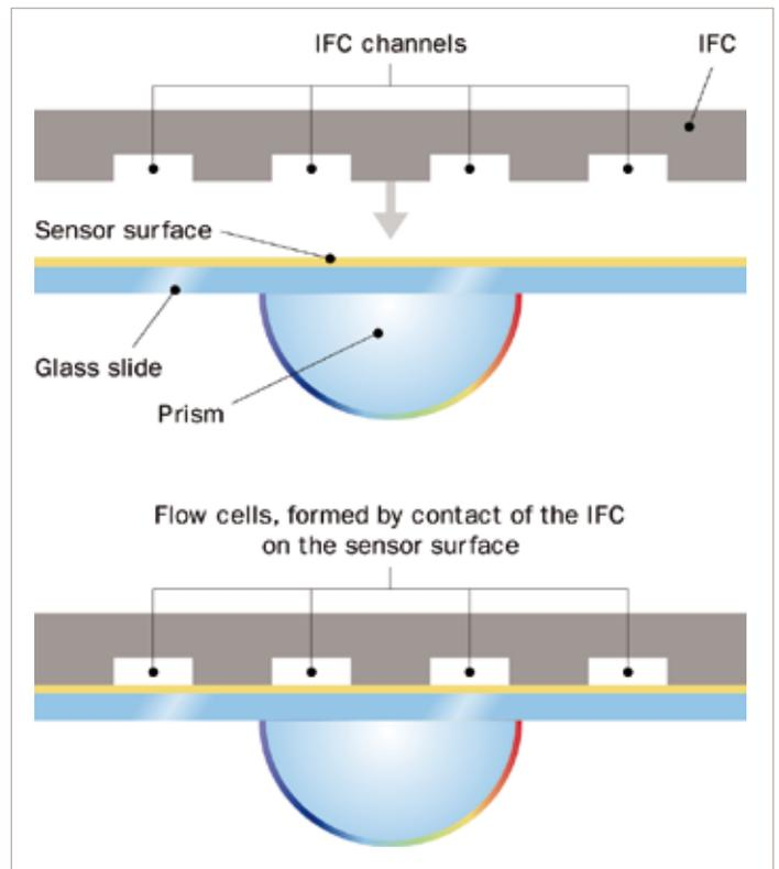
**Figure 4A.** Flow cells are formed in prism-based SPR detection by pressing an integrated microfluidic cartridge (IFC) against a sensor surface - the site of interaction on which one partner is immobilized and over which the other passes during sample injection.
