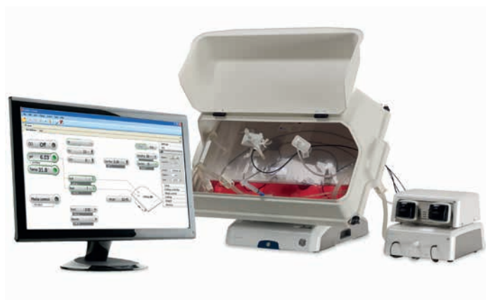
Fig 1. ReadyToProcess WAVE 25 bioreactor system comprises a rocker, a gas mixer, and a pump unit, all operated by the UNICORN™ software installed on a client computer. The rocker has multiple functions, including heating, culture mixing, and weight measurement. The gas mixer delivers gas of a defined composition to the culture and is used together with optical sensors in the Cellbag™ bioreactor for online control of culture pH and DO. Liquid is delivered to the culture by the pump unit, which supports a range of flow rates to cover multiple applications, from addition of feeds or base to perfusion culturing. The system can also be controlled by an external control system such as the Emerson DeltaV™ using the UNICORN open platform communication (OPC) server.
