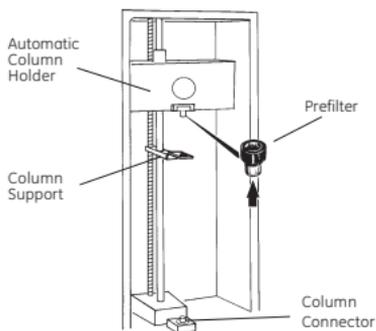
**Fig 1.1.** Check that the Automatic Column Holder is high enough to install the column. It is recommended to use Prefilter 0.8 mm or 3.2 mm (Code No. 18-1800-75 and 18-1800-76) to protect the column.
