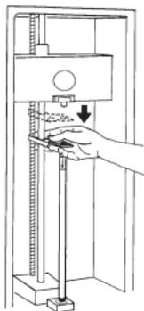
**Fig 1.3.** Align the column vertically with the Column Support.
