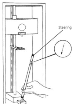
**Fig 1.2.** Put the column onto the Column Connector. The arrow on the label, which indicates the correct flow direction, should point downwards.
