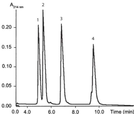
Fig 2. Function test for  $\mu$ RPC C2/C18 SC 2.1/10.
