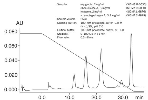
**Fig 1.** Typical chromatogram from a function test of SOURCE 15PHE PE 4.6/100.
