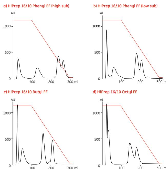
**Figure 1.** Typical chromatogram from a function test of (a) HiPrep 16/10 Phenyl FF (high sub), (b) HiPrep 16/10 Phenyl FF (low sub), (c) HiPrep 16/10 Butyl FF and (d) HiPrep 16/10 Octyl FF.
