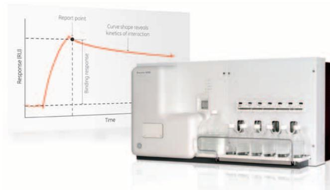
Biacore system sensorgrams define whether binding takes place at all and if so to what extent. The sensorgram also shows in real-time how fast the binding and dissociation takes place. Equations can then be fitted to the resulting curve to calculate on rates, off rates, and affinities.
