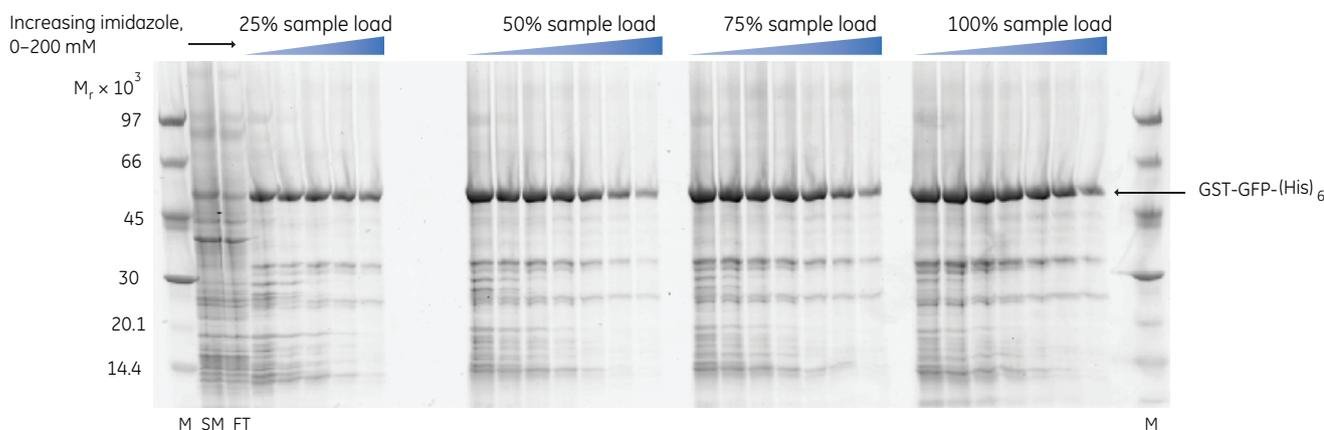
**Fig 4.** SDS-PAGE of GFP-(His)<sub>6</sub> enriched from a background of *E. coli* protein using His Mag Sepharose Ni beads. GFP-(His)<sub>6</sub> was detected using Deep Purple™ Total Protein Stain and Ettan™ DIGE Imager. The gel image was analyzed with ImageQuant™ TL software. M = molecular weight markers, SM = start material, FT = flowthrough from a sample load of 75% of the total binding capacity, 40 mM imidazole.
