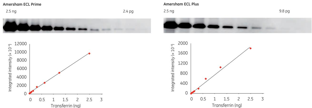
**Fig 1.** Western blotting detection of transferrin in a two-fold dilution series using Amersham ECL Prime (left) and Amersham ECL Plus (right). The samples were blotted on to an Amersham Hybond-P (PVDF) membrane and imaged using an ImageQuant LAS 4000 mini system.
