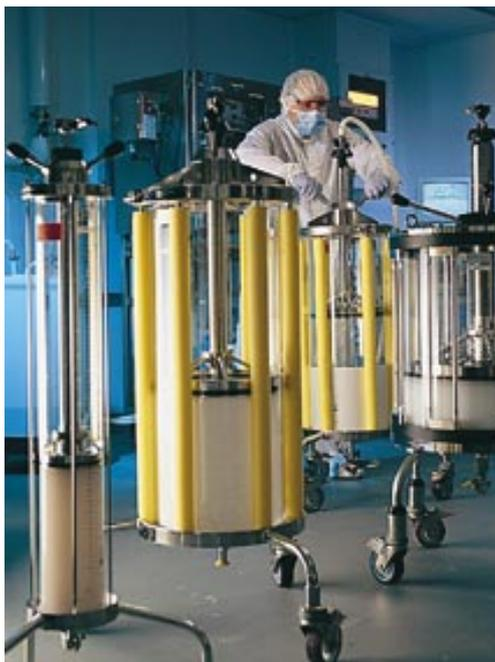
BPG columns are used by Hybridon Inc. in the manufacture of oligonucleotides. BPG columns are glass columns designed for biopharmaceutical production. They are available in a range of dimensions and volumes. Photo courtesy of J. Kannair.
