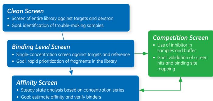
**Fig 5.** Typical SPR FBDD workflow. Biacore 4000 and Biacore S200 have dedicated functionality for running and evaluating **Clean Screen**, **Binding Level Screen**, and **Affinity Screen** (shown in blue). In addition, Biacore S200 provides support for running **Competition Screen** cost-effectively and rapidly (shown in green).
