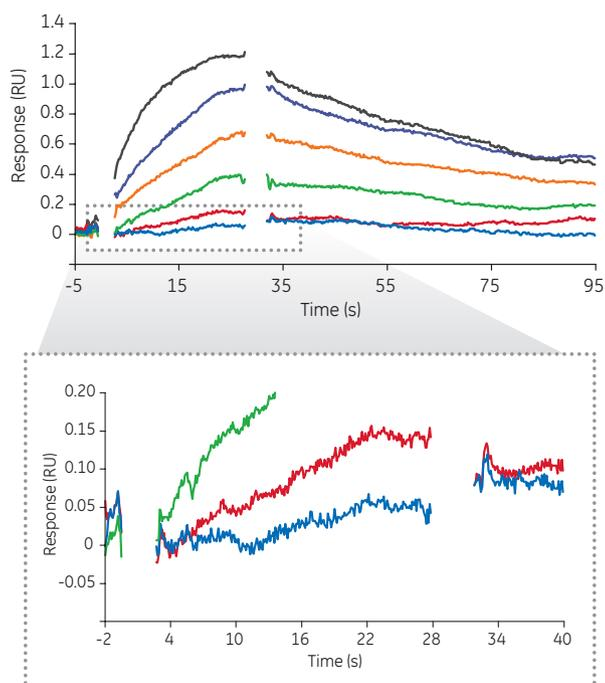
**Fig 4.** The high sensitivity of Biacore S200 enables confident analysis of data even in the sub-resonance units (mRU) response range. This means low density surfaces can also be used for targets with limited activity. Upper graph: Sensorgram from a kinetic experiment between thrombin and melagatran. Lower graph: Zoom-in on the lower concentrations demonstrating the possibility to separate curves at sub-resonance response levels.
