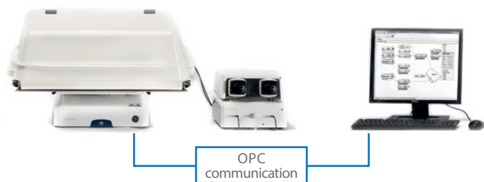
Fig 9. Setup of the WAVE 25 Bioreactor System on a client PC with DeltaV.
