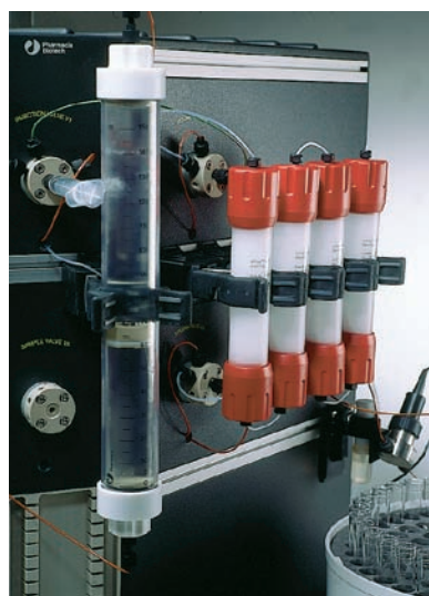
Fig 11. Four HiPrep 26/10 Desalting columns connected in series.
