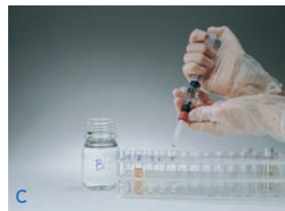
Fig 2. Syringe operation of HiTrap Protein G HP 1 ml.
