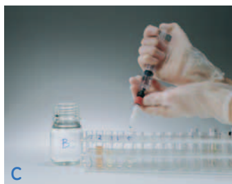
Figure 2. Using HiTrap rProtein A FF, HiTrap Protein A HP or HiTrap Protein G HP with a syringe.
