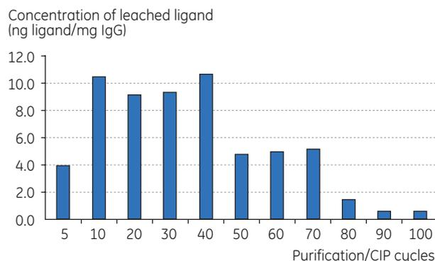
**Fig 4.** Ligand leakage (ppm) of MabSelect SuRe over 100 cycles of CIP in conjunction with the purification of humanized IgG<sub>4</sub>. Cleaning-in-place was performed with 0.1 M NaOH and the contact time was 15 min/cycle.
