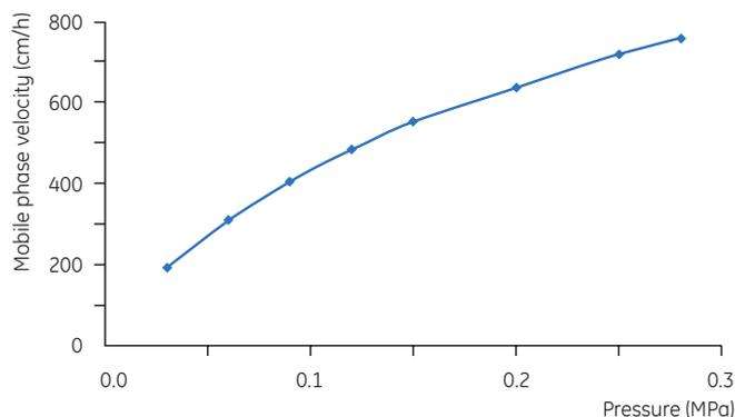
**Fig 9.** Pressure/flow profile for MabSelect SuRe in a packed bed (bed height 20 cm) in a BPG 300 column (i.d. 300 mm).
